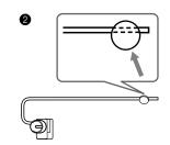
Affix the antenna with a thumbtack. (Do not push the thumbtack *through* the antenna.)
